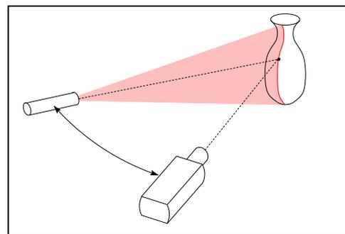
*Fig.1. Conventional single-camera light stripe sensor*
