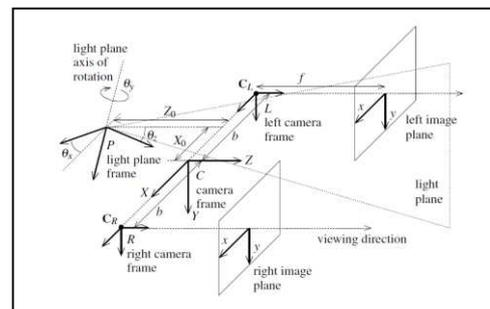
Fig.4. Light stripe camera system model
