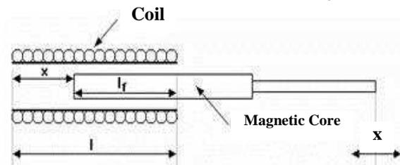
Fig.2. Inductive sensor with mobile core with the same length as the coil.
