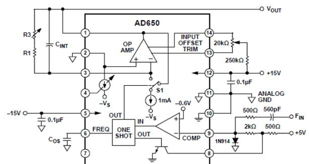
Fig.6. The f to V converter
