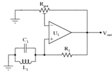
Fig.5. Oscillator circuit inductive transducers.
