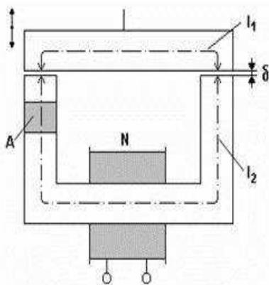
Fig.1. Inductive sensor with mobile “I” core
