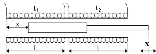
Fig.3. Inductive transducer with differential coils
