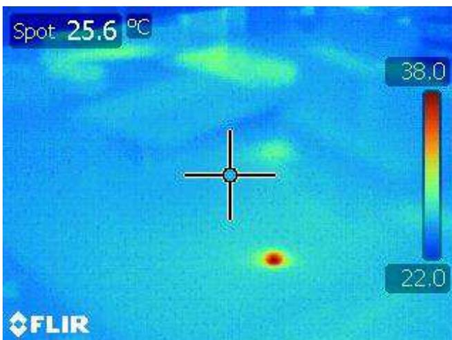
Figure 4. Thermogram of a shining porcelain table which reflects radiation of other objects
