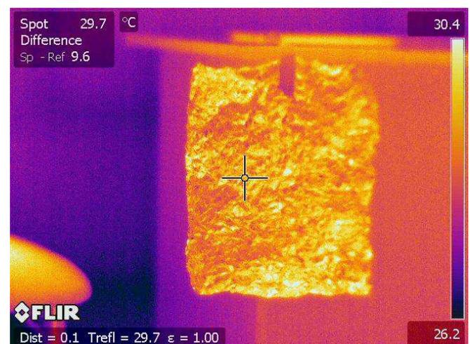
Figure1. Thermogram taken with Flir Systems ThermoCam B620 of an aluminum foil which reflects thermal radiation [3]
