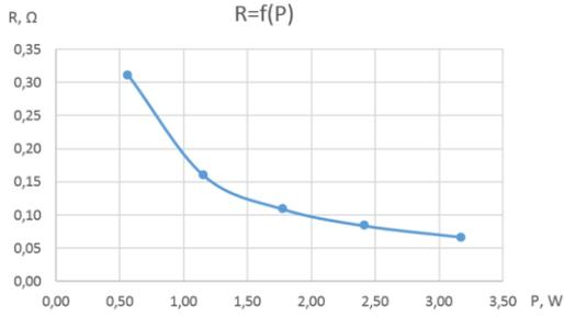
Figure 3. The optimal load resistance depending on the irradiance
