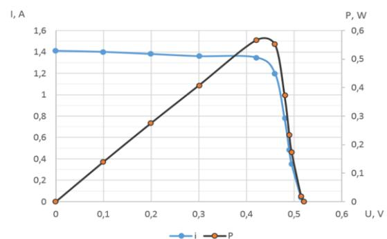
Figure 2. VA characteristics of the photovoltaic cells at irradiance of 200 W/m<sup>2</sup>
