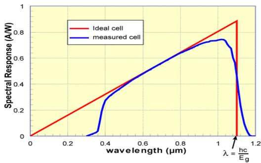
Figure 4. Spectral response of the silicon photovoltaic cell
