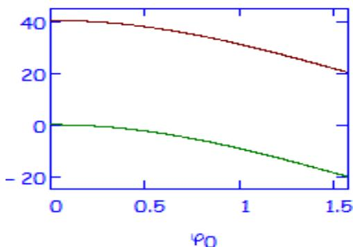
Figure 5 Maximum and minimum values of the stator current for initial values of the angle  $\varphi_0 = 0 \dots \pi/2$ , max (brown), min (green)
