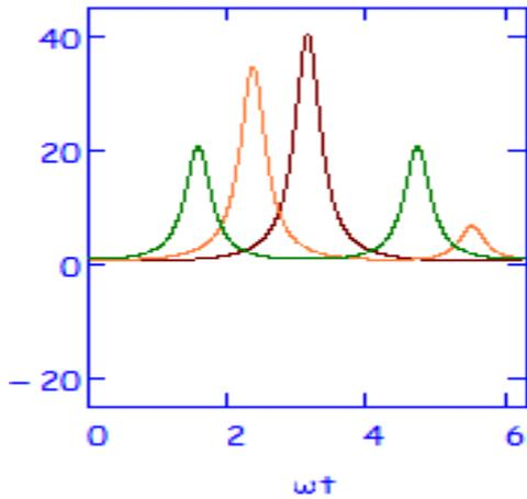
Figure 4 Current propagation in rotor depending from the entry of the short circuit with  $\varphi_0 = 0$  (brown),  $\varphi_0 = \pi/4$  (orange),  $\varphi_0 = \pi/2$  (green)
