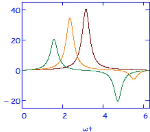
Figure 3 Current propagation in stator depending from the entry of the short circuit with  $\varphi_0 = 0$  (brown),  $\varphi_0 = \pi/4$  (orange),  $\varphi_0 = \pi/2$  (green)
