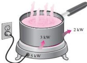
Figure 4 The efficiency of a cooking appliance represents the fraction of the energy supplied to the appliance that is transferred to the food
