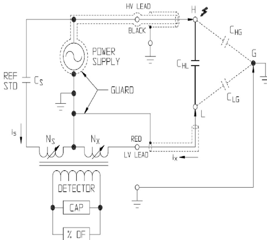
Figure 1. Simplified scheme for determining tgδ using a Delta-2000 kits
