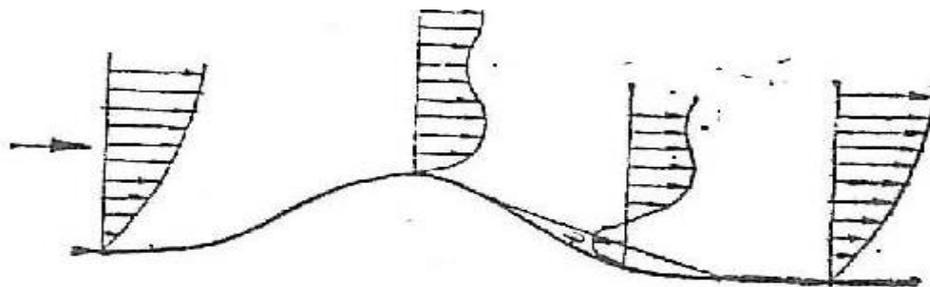
Figure 1. The distribution of wind speeds at a well rounded hill
