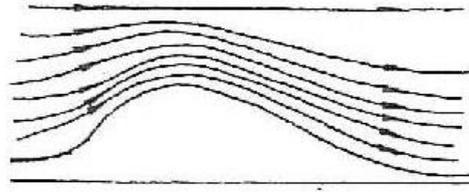
Figure 2. The effect of accelerating the wind speed of a hill sloping
