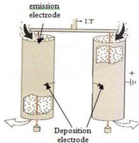
Figure 7 - The gas inlet in a tubular electrofilter.
