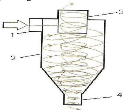
Figure 2 - Circuit diagram of a cyclone: 1-raw gas inlet connection, 2-cylindrical casing, 3-pipe exhaust cleaner, 4-pipe dust extraction
