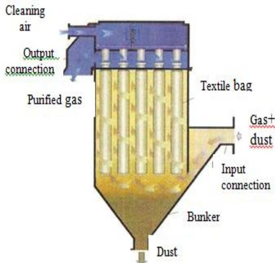
Figure 3. - The principle of a bag filter
