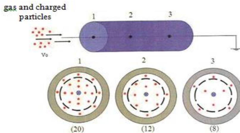
Figure 5 - Schematic representation of a simple electrostatic precipitator.
