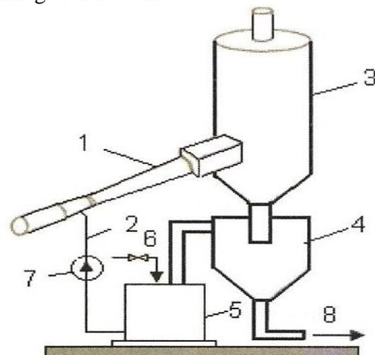
Figure 4.- A schematic diagram of a sewage treatment plant with a nozzle tube diffuser Venturi, 2-water injection, 3-cyclone, 4-sedimentation vessel, 5 water tank, 6-water addition, 7 - pump, 8-sludge
