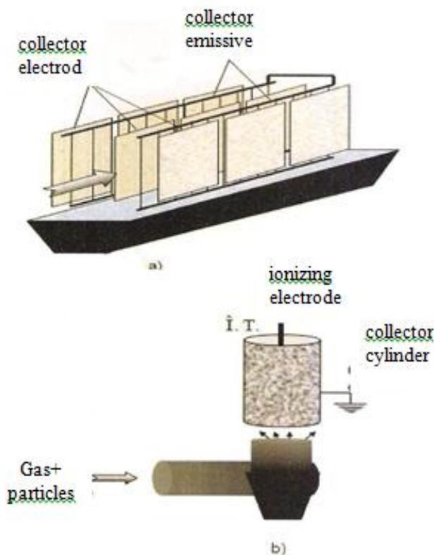
Figure 6 Schematic view of an electrostatic filter:
