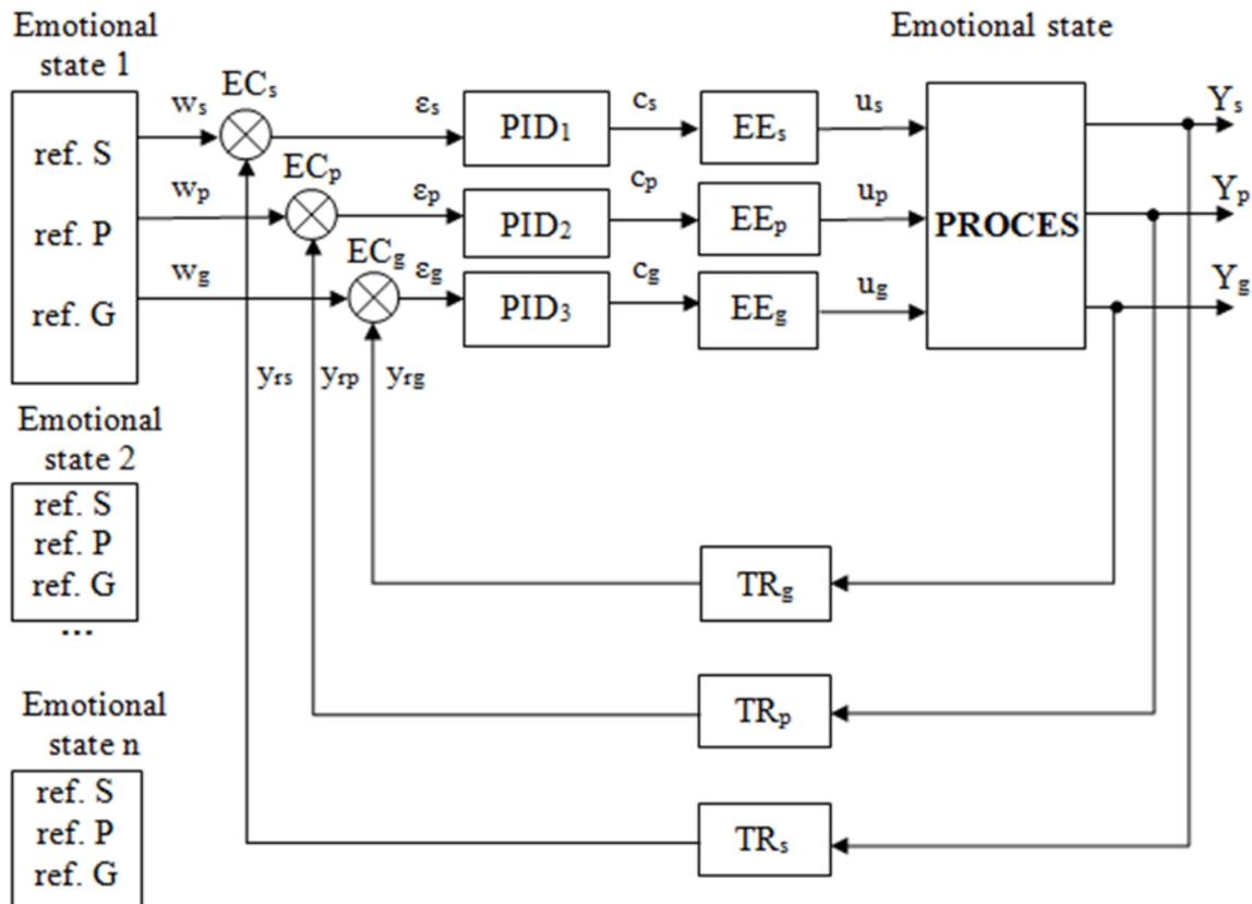
Figure 7. Block diagram for command and control of the biomimetic structure
