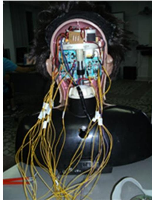
Figure 5b). The mechanical and electronic structure Robot ELVIS
