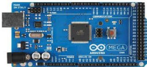
Figure 6. The ARDUINO MEGA board
