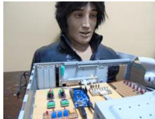
Figure 5c). The electronic structure for control and command Robot ELVIS
