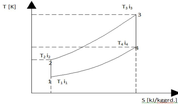
Figure 2. The theoretical diagram of the open-circuit gas turbine
