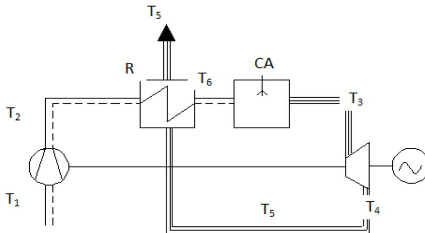
Figure 3. Preheating of the air by heat recovery: R - recuperator preheater; CA-combustion chamber
