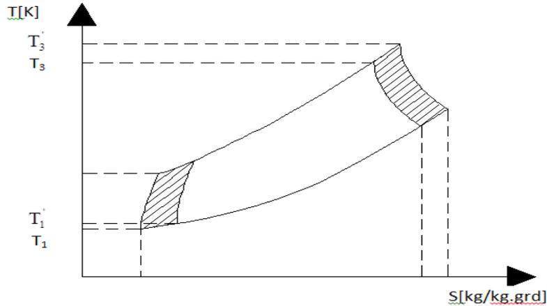
Figure 4. The effect of lowering the suction and lifting temperature of the final temperature
